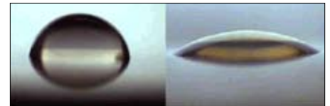
Figure 10. Water droplets in contact with a nylon surface before (left) and after UV surface exposure.
