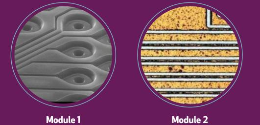
Module I Micro-patterned polymer surface **Module 2** 50µm wide silver tracks printed on polymer
